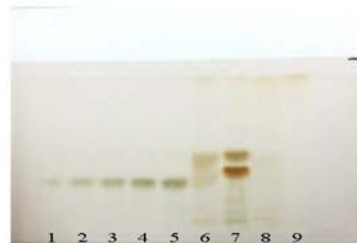
Figure 5: A comparative TLC profile of Maltose along with different plant parts of L. scindicus (Track 1-5 Maltose concentrations and tracks 6 (HML), 7 (HMS), 8 (HMI), 9 (HMR) respectively
